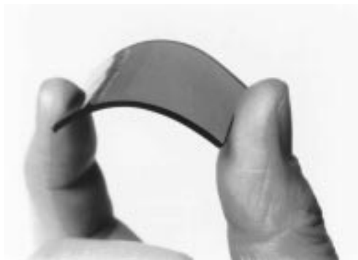
Fig. 2 Photograph of a Ti-O-PDMS hybrid. The molecular mass of PDMS was 3000. Heat treatment was performed at 150 °C for 72 h.
